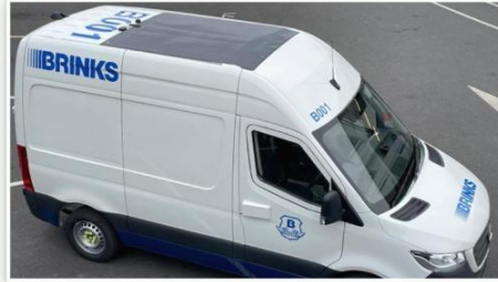
Vehicle solar panels projected to save 580 liters of fuel and reduce 1.5 metric tons of CO2 emissions, per vehicle, per year
